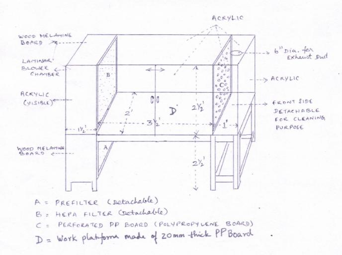
Note: Width of the Laminar blower chamber may be vary (given 1<sup>1</sup>/<sub>2</sub>') depends upon the blower assembly during manufacturing.
